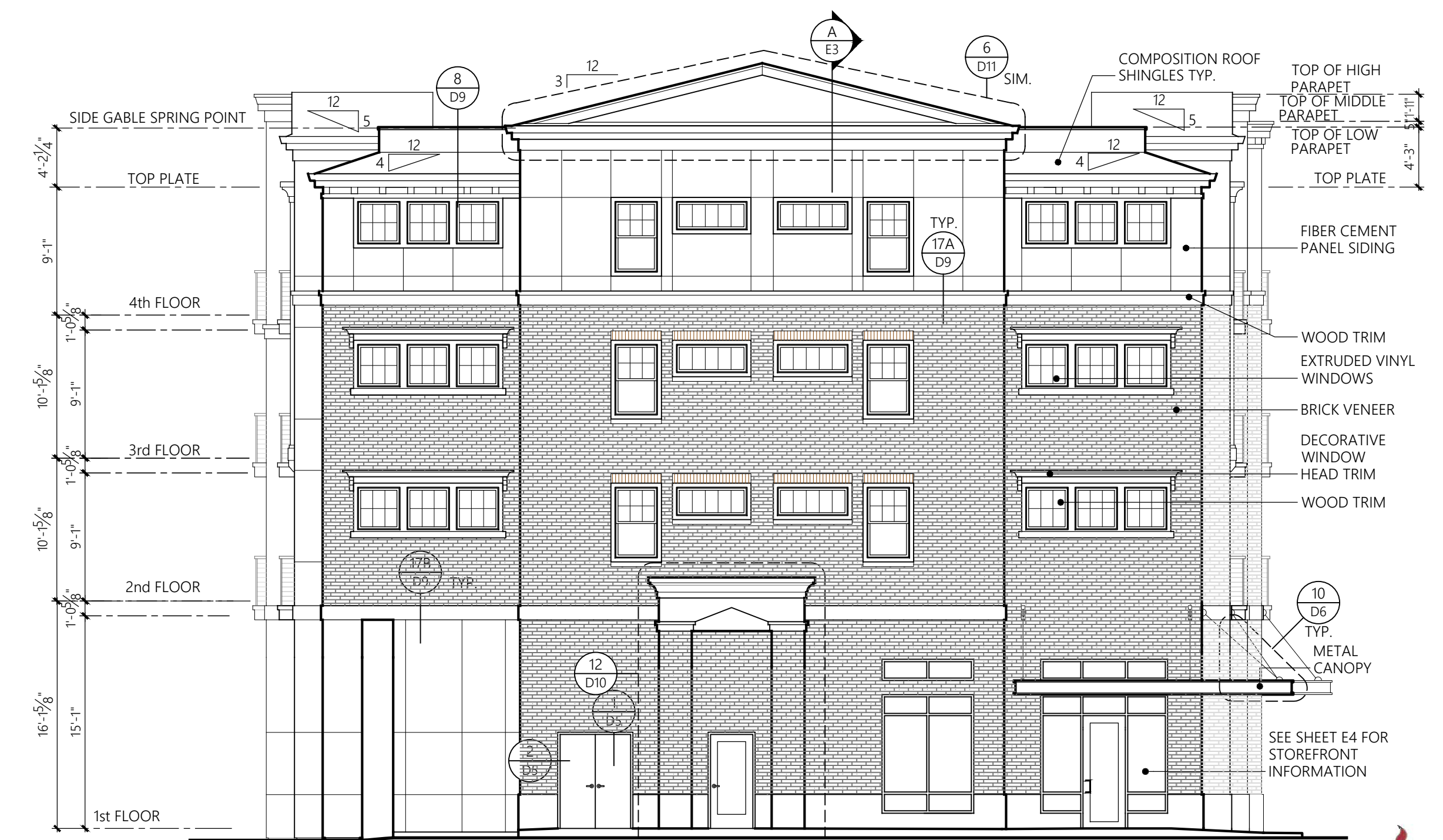
Buildings 1, 2, 7 & 8 SIDE ELEVATION 1/8" = 1'-0"
